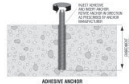
Figure 110: Adhesive anchor installation.
