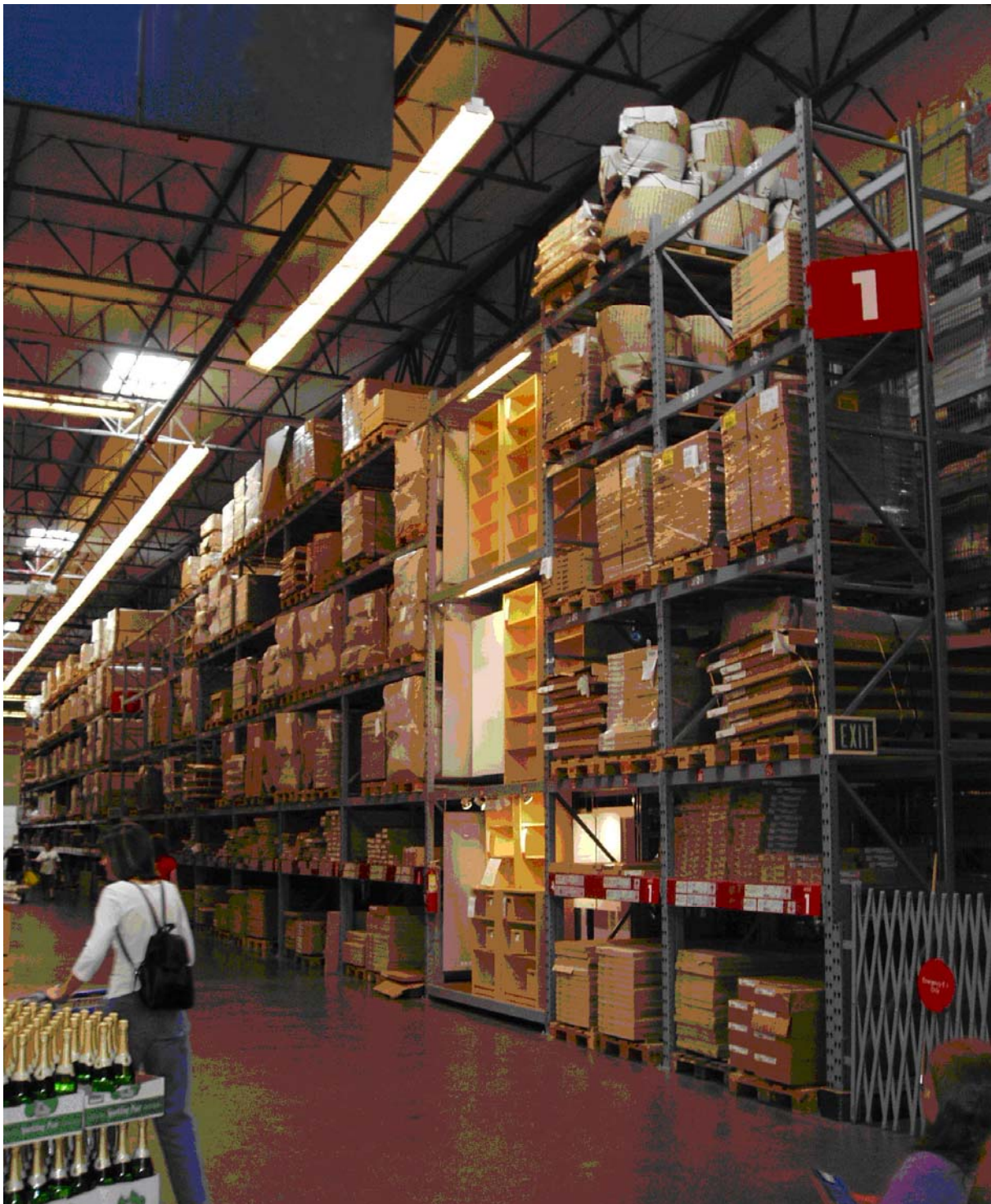
Figure 8-1 Rack contents on racks should be adequately restrained to prevent their falling into aisles.
