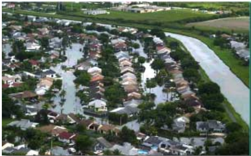
Residential flooding caused by rising water table, reflected in height of water in canal. Recharging of the aquifer immediately below the surface has exceeded the canal systems discharge capacity to move the excess water to the ocean and to the Everglades. Pumping and dredging will improve the canal conveyance capacity.
