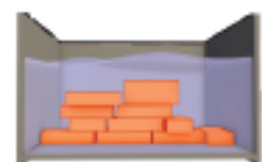
Bricks are soaked in water before use
