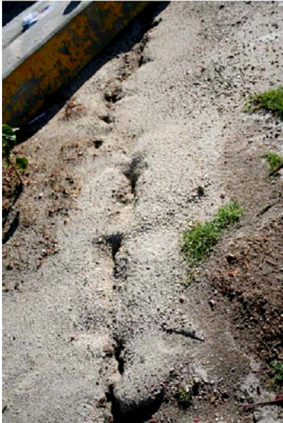
Figure 3.15. Sand boils at Kawaihae Harbor from the 2006 Hawaii Earthquakes [UHM].
