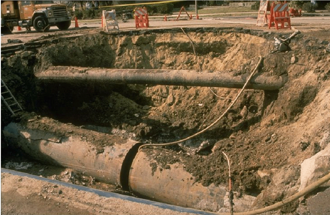
Figure 3.42. Utility pipe ruptured by lateral spreading on Balboa Boulevard from the 1994 Northridge Earthquake [NISEE].
