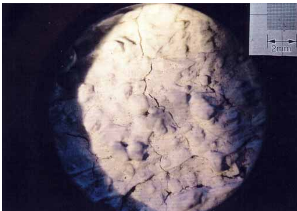
Figure 5.8. Magnified crazing cracking (not earthquake damage) in stucco – circle is 5/8-inch across; bumps are grains of sand in stucco texture [Exponent].
