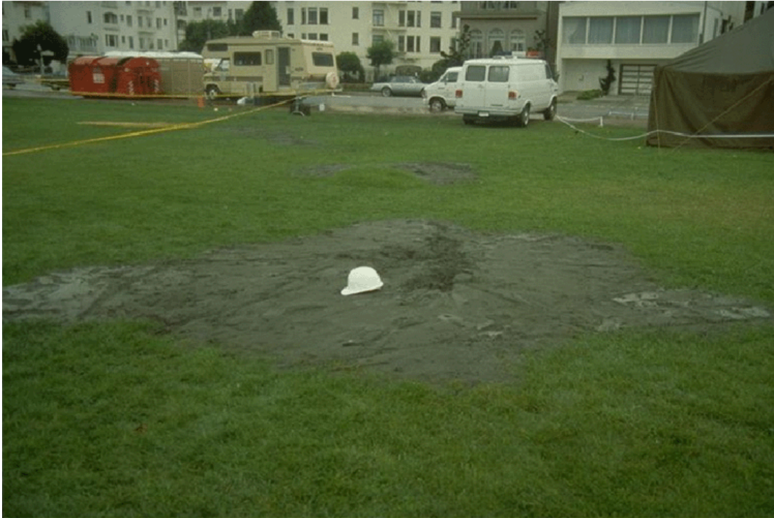
Figure 3.13. Sand boil due to liquefaction of old, poorly compacted, water-saturated fill during the 1989 Loma Prieta Earthquake [NISEE].
