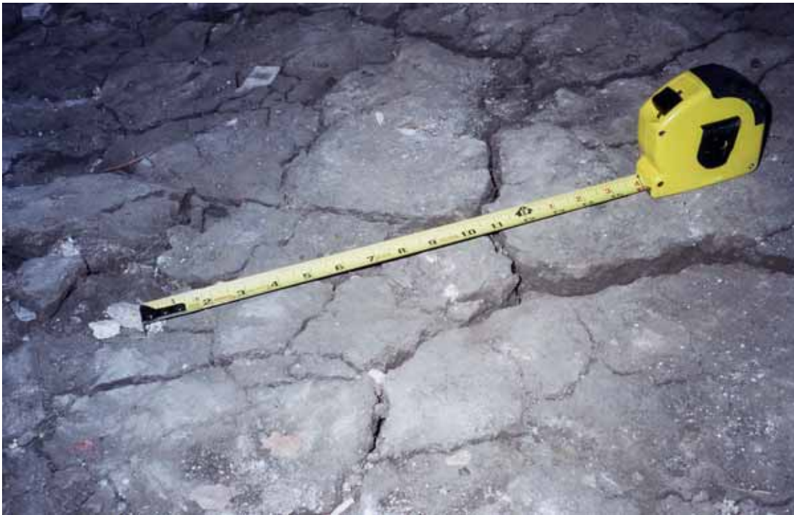
Figure 3.6. Desiccation cracking of expansive soil within a crawlspace, a long-term, non-earthquake condition [Exponent].
