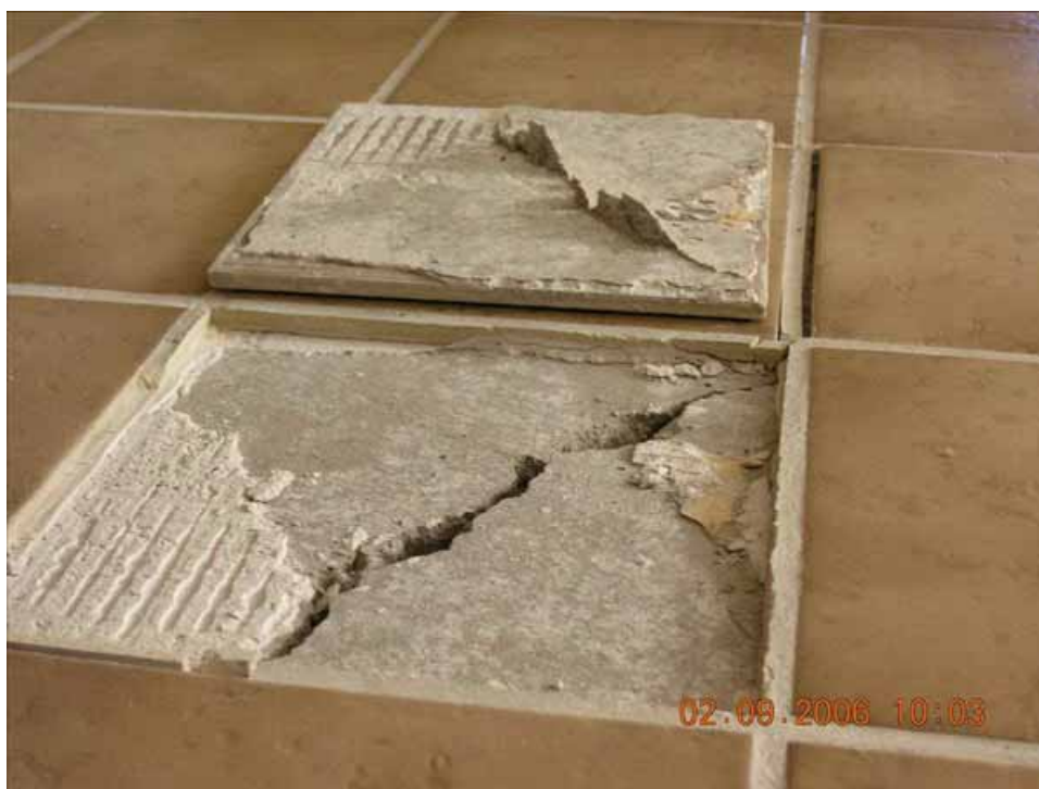
Figure 4.36. Setting mortar that had flowed into an existing slab crack that remained bonded to the backside of a ceramic tile when the tile was removed, a clear indication that the concrete slab was cracked when the tile was installed [Exponent].
