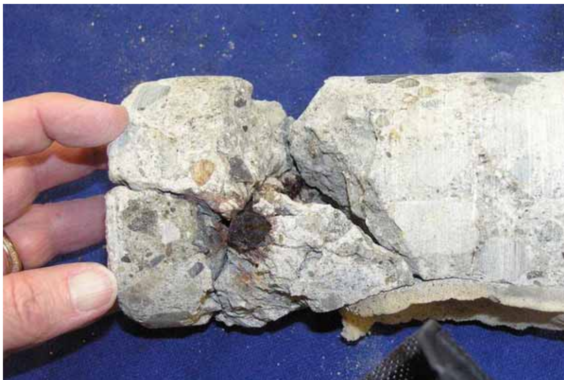
Figure 4.12. Core extracted from concrete stem wall showing cracking caused by swelling pressure generated by corroding reinforcing steel [Exponent].
