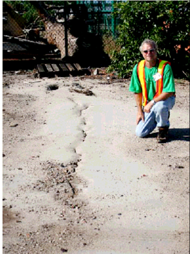
Figure 3.15. Sand boils at Kawaihae Harbor from the 2006 Hawaii Earthquakes [UHM].
