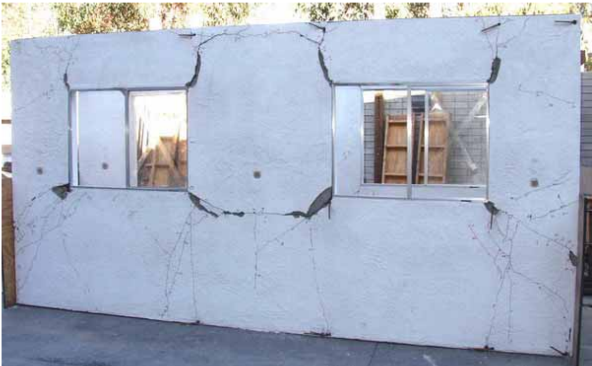
Figure 5.12. Severe cracking and spalling of stucco wall test specimen after earthquake load testing [Exponent].
