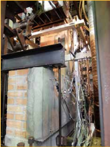
Figure 4.2.6. Jacketing (reinforcement concrete panel)
