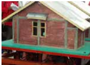
Detail of 1/10 scale model house of confined brick masonry
