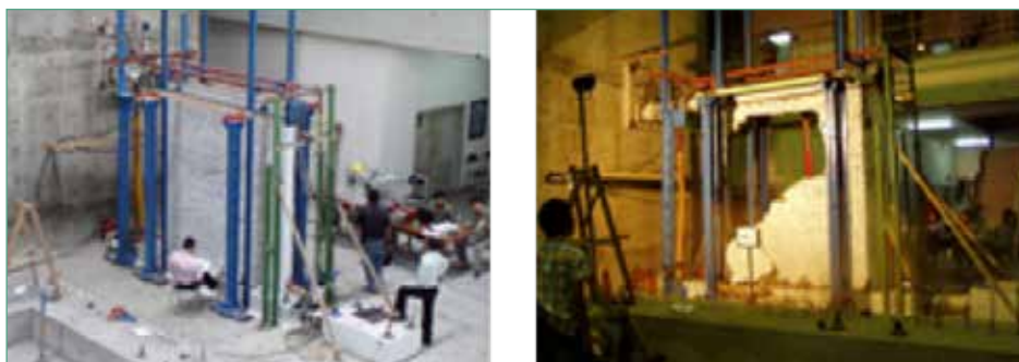
Figure 1.1.12 Cyclic loading experiments of confined masonry walls (9 specimens), February and March 2009, at the Research Institute for Human Settlements, Department of Public Works (RIHS/DPU), Bandung, Indonesia, organized by Bandung Institute of Technology (ITB) and BRI. Setting up of specimen- and measurement equipment (left), and final stage of cyclic loading (right)
