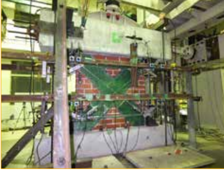
Figure 4.2.6. Jacketing (reinforcement concrete panel)
