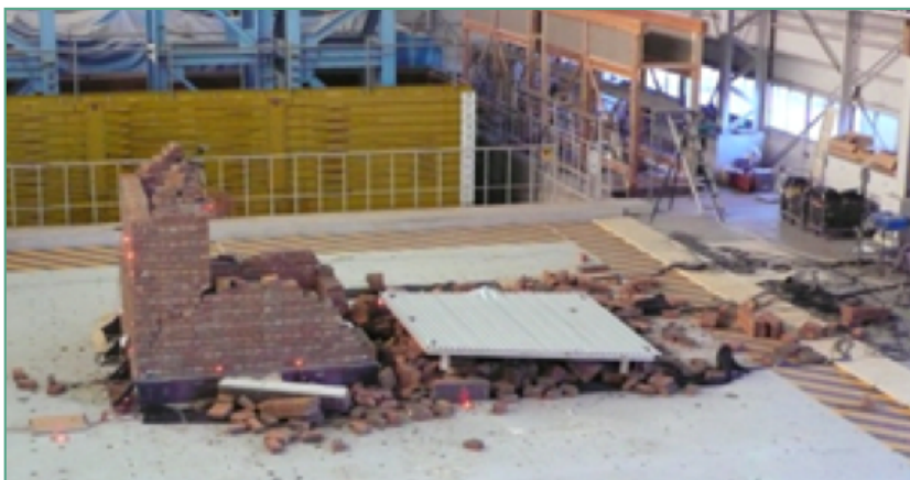
Figure 4.1.5. Model structure after shaking
